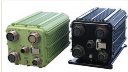
Figure 2 | The EFV program influenced the development of the COTS DuraMAR 3230 subsystem, which has only minor mechanical differences from the TSR and will become a standardized version of the TSR for generalized use by the armed forces.
