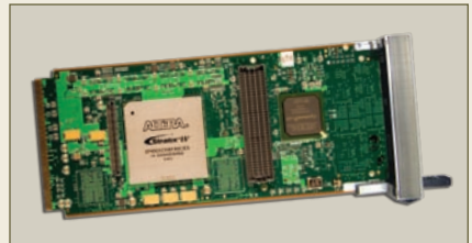
Figure 2 | Vendors such as BittWare are putting FMC sites on their boards. Pictured: An Altera Stratix IV based AMC.
